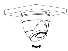
Fix the pedestal by drilling locking holes around the sticker and inserting three expansion bolts into the holes and fastening it with three locking screws.
