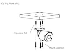
Insert three expansion bolts in place into the ceiling and fix the equipment with three mounting screws.
