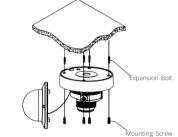
Use the position indicated on the position sticker to drill the holes needed to mount the camera base. Insert the expansion bolt into the holes. Match the base's mount openings to the expansion bolts position, then place the mounting screws through the base's mount opening into the expansion bolt. Tighten the mounting screws to ensure the camera base mounted securely.
