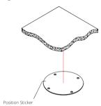
Apply the position sticker to the desired camera mounting position.
