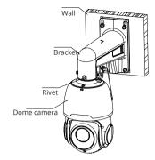
Step 5: After the tail cable of the dome camera passes through the bracket, align the notch of the adapter cover with the rivet position of the bracket and insert it into the bracket hole.
