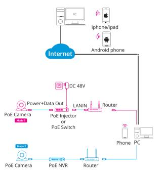
**A**ttention:There are two connection modes: 1. For non-PoE router, pls connect the camera by a PoE switch or a PoE injector.
