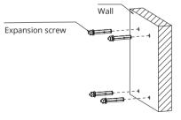
Step 2: Hammer the 4 expansion screws into the drilled wall holes.
