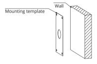
Step 1: Stick the mounting template to the wall, drill 4 expansion screw holes.
