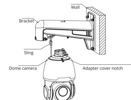
Step 4: Fasten the anti-dropping rope of the locked dome camera into the suspending rope loop of the bracket.
