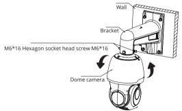
Step 6: After rotating the dome camera to the proper position, tighten the 2 socket head cap screws M6\*16 on the bracket.
